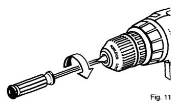
Insert allen wrench in chuck and tighten chuck jaws securely. Tap sharply with a mallet in a counterclockwise direction. This will loosen chuck on the spindle. It can now be unscrewed by hand. See Figure 12.
